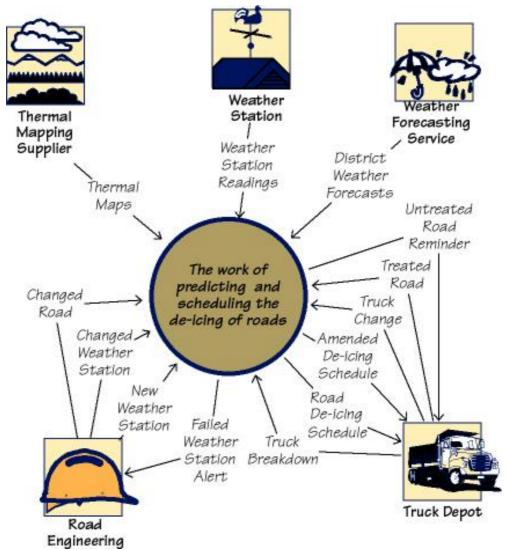
This work context model defines the connections between the part of the world that is under investigation and other people, organizations, hardware and software (referred to as adjacent systems). The inputs and outputs represent the data and material that travels between the work and other parts of the world. The work context is the basis for partitioning the investigation and discovering the requirements.
